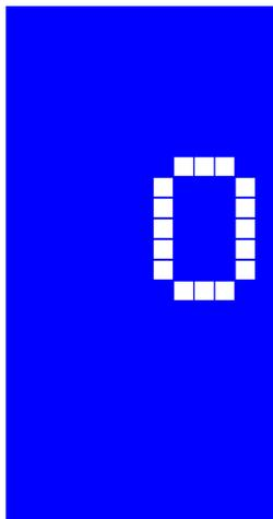
Here right char blinks. Now it can be changed by pushing INC (↑) and DEC (↓) buttons. Any number or letter can be chosen. After selecting right char push ENT shortly and left char starts to blink. In the same way left char is set.
