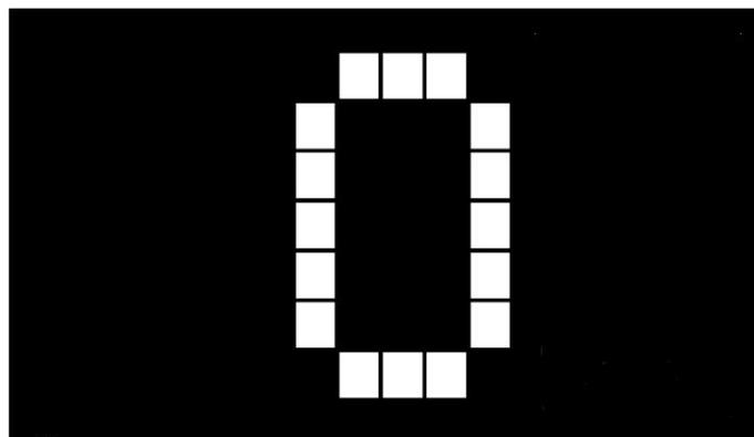
Here right char blinks. Now it can be changed by pushing INC (↑) and DEC (↓) buttons. Any number or letter can be chosen. After selecting right char, push ENT shortly and left char starts to blink. In the same way left char is set. Then select floor and signal color by pushing ENT and change with INC (↑) and DEC (↓) buttons. If no color selected to signals, then floor color displays.
